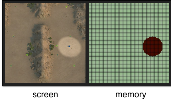
Figure 4. Memory representation of a visibility map structure
