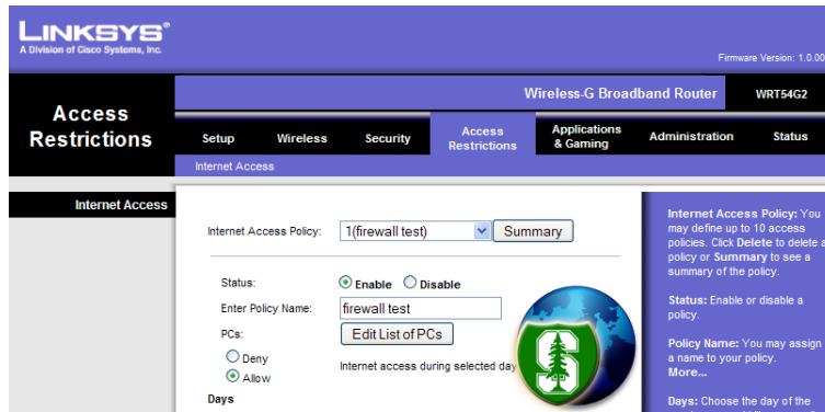
Figure 21: An XSS attack in an access restrictions field that embeds the Stanford Security Lab logo.
