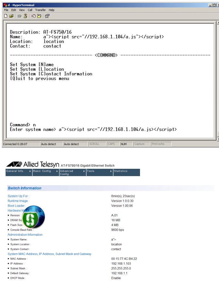
Figure 12: The console showing how to carry out the XCS attack and the result of the console XCS attack.
